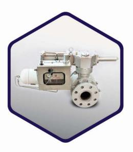
PEPCO pressure protection system is designed to protect equipment downstream of a pressure reducing station. it consists of a complete ball valve with actuator and control system supplied in a self-contained and compact unit. it should be installed in upstream of the stations. if there is an excessive change in pressure downstream, it will react by shutting off the gas supply; the pressure switch can sense either rising pressure, falling pressure or both as specified.
