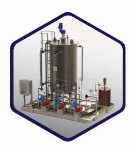
In this industry, responsibility of this package is to inject corrosion/Asphaltene inhibitor from its storage tank into the pipeline, continuously. The dosing pumps are most important equipment in this package; Mixer, Storage tank, control system, pulsation damper, calibration pot, pressure gauge and level gauge Can use in such packages as needed.
