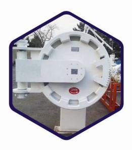
All filtration equipments are enclosed with Quick Opening Closure, which all stages of construction, including mechanism design, mechanical analysis, machining and assembly, are performed in this complex. PEPCO has the ability to manufacture such doors in an any type, including Hub & Clamps, Bayonet, Yoke and Band Lock, and in accordance with the latest eddition of the IPS and IGS Standard and ASME/API codes.
